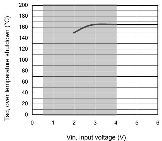
**Figure 14 – Over temperature shutdown (°C)
