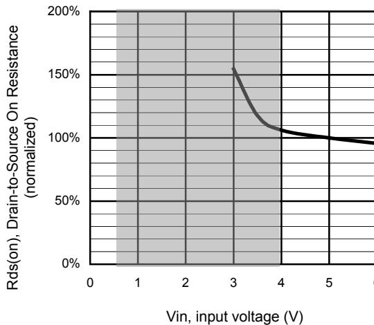
Figure 5 – Normalized R<sub>dson</sub> (%) Vs Input voltage (V)
