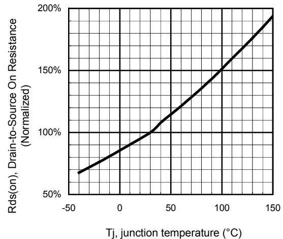
Figure 6 - Normalized R<sub>dson</sub> (%) Vs T<sub>j</sub> (°C)
