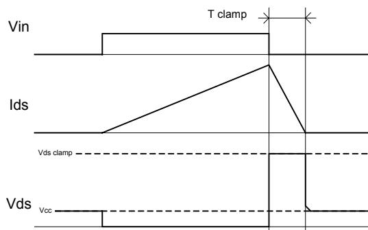
Figure 3 – Active clamp waveforms
