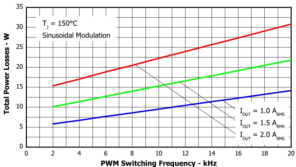
Figure 5. Total Power Losses vs. PWM Switching Frequency, Sinusoidal modulation
