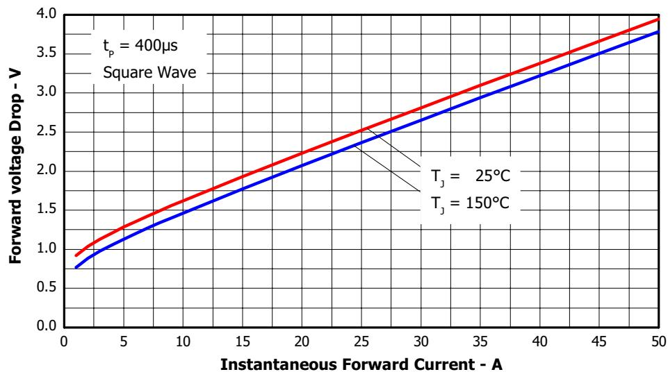
Figure 11. Maximum Forward voltage Drop (Input Bridge Rectifier)
