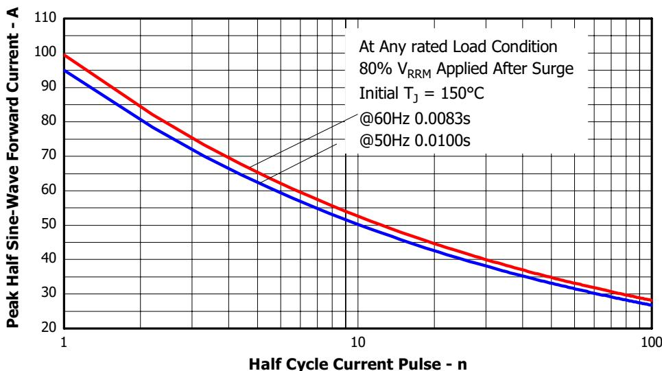
Figure 14. Input Bridge Maximum Non-Repetitive Surge Current
