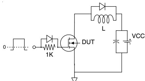
**Fig 19a.** Gate Charge Test Circuit
