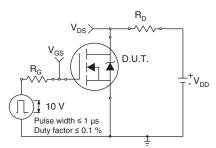
Fig. 10a - Switching Time Test Circuit
