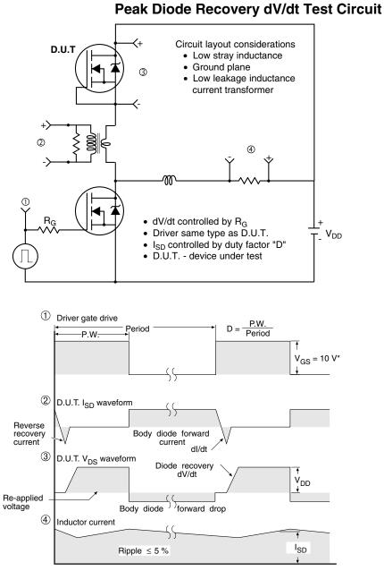
\*  $V_{GS}$  = 5 V for logic level devices
