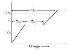
Fig. 13a - Basic Gate Charge Waveform
