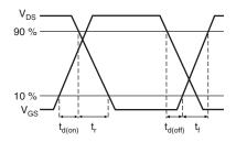
Fig. 10b - Switching Time Waveforms
