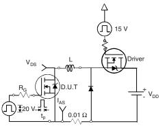
Fig. 12a - Unclamped Inductive Test Circuit
