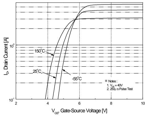
**Figure 2. Transfer Characteristics**
