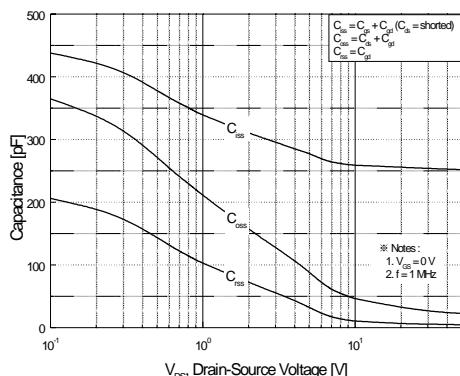
**Figure 5. Capacitance Characteristics**
