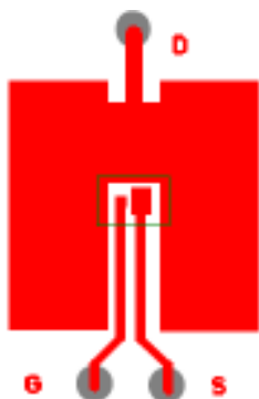
① Surface mounted on 1 in. square Cu (still air).
