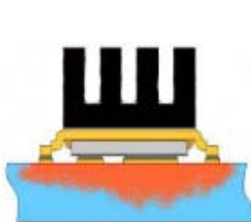
② Mounted to a PCB with small clip heatsink (still air)
