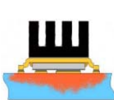
⑨ Mounted on minimum footprint full size board with metalized back and with small clip heatsink. (still air)
