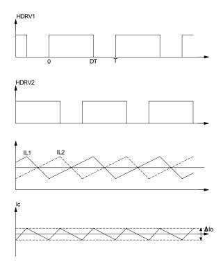
Fig. 4: Current ripple cancellation for output
