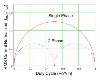
Fig. 5: Input RMS value vs. Duty Cycle
