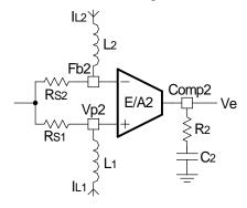
Fig. 21: The Compensation network for current loop
