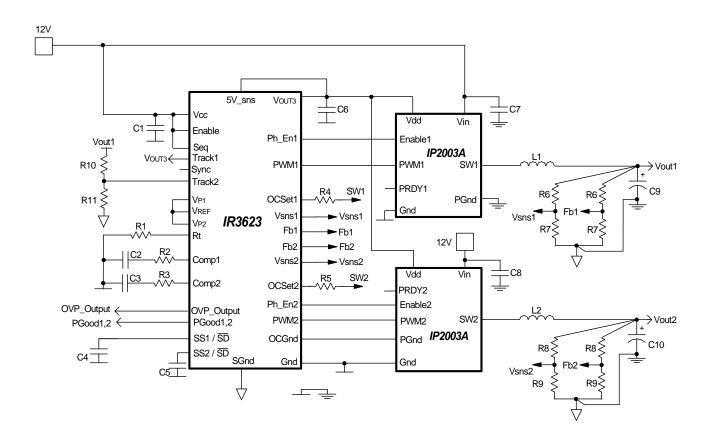
Fig. 23: Application circuit for Dual output application Tracking and sequencing using Track pin
