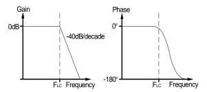
Fig. 18: Gain and Phase of LC filter
