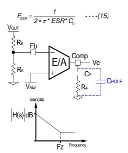
Fig. 19: TypeII compensation network and its asymptotic gain plot
