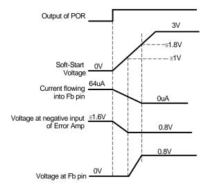
Fig. 8: Theoretical operation waveforms during soft-start
