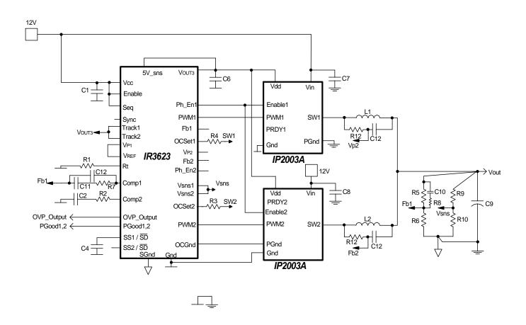
Fig. 22: Application circuit for 13.2V to 1.8V @ 40A
