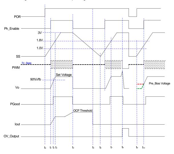
Fig. 12: Fault Conditions
