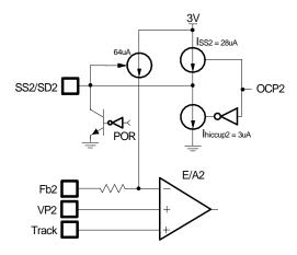
Fig. 7: Soft-Start circuit for IR3623
