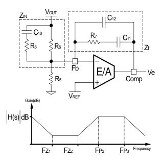
Fig. 20: Compensation network with local feedback and its asymptotic gain plot
