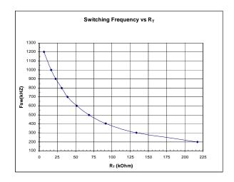
Fig. 16: Switching Frequency vs. External Resistor (R<sub>t</sub>)
