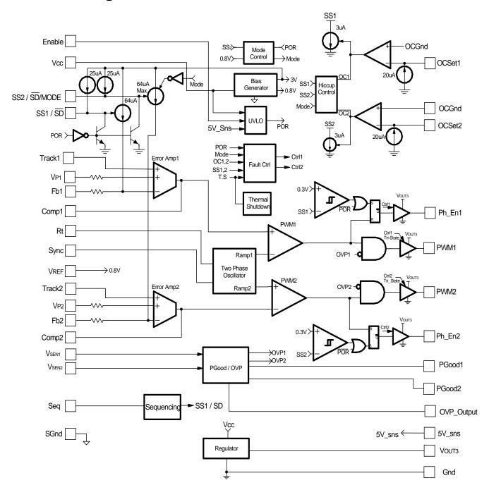
Fig. 2: Simplified block diagram of the IR3623
