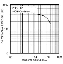
DC FORWARD CURRENT GAIN VS. COLLECTOR CURRENT
