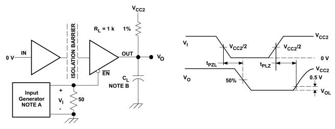
Figure 3. ISO722 Sleep-Mode Low-Level Output Test Circuit and Voltage Waveforms
