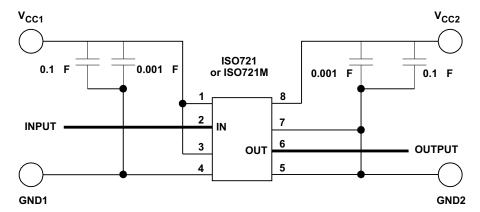
Figure 18. Basic Application Circuit
