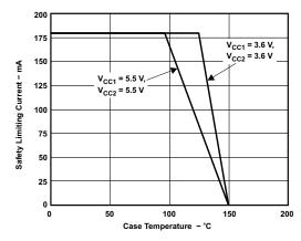
Figure 7.  $\theta_{\text{JC}}$  THERMAL DERATING CURVE per IEC 60747-5-2
