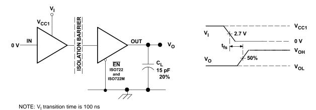
Figure 4. Failsafe Delay Time Test Circuit and Voltage Waveforms
