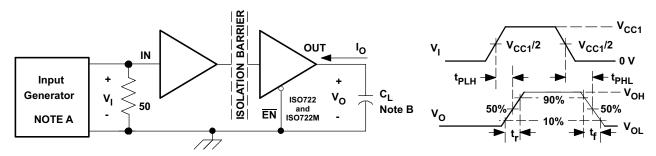
Figure 1. Switching Characteristic Test Circuit and Voltage Waveforms
