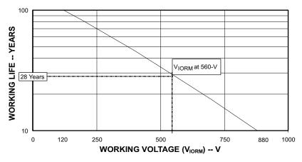
Figure 14. Time Dependant Dielectric Breakdown Testing Results
