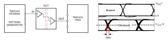
NOTE: PRBS bit pattern run length is 2<sup>16</sup> – 1. Transition time is 800 ps. NRZ data input has no more than five consecutive 1s or 0s.
