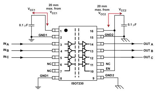
Figure 13. Typical ISO7230 Application Circuit
