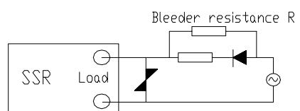
Note: Connect bleeder resistor R.
