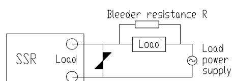
Note: connect bleeder resistor R.
