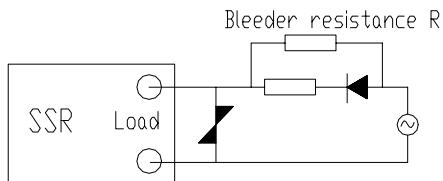
Note: Connect bleeder resistor R.
