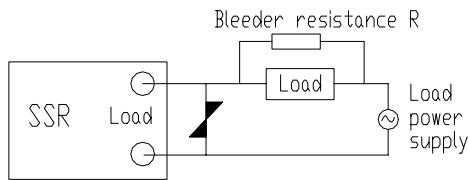
Note: connect bleeder resistor R.
