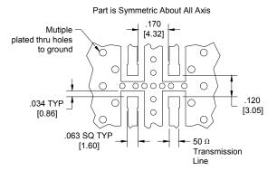
Dimensions are in Inches [Millimeters] JP506 Rev A Mounting Footprint
