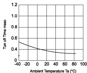
**Fig.5** LED operate vs. ambient temperature
