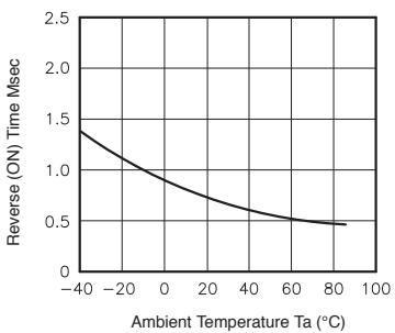
**Fig.5** LED operate (ON) vs. ambient temperature
