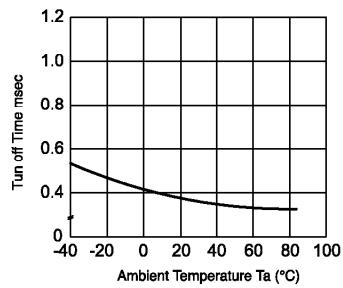
**Fig.5** LED operate vs. ambient temperature
