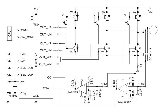
Note 1: Take enough care in designing output  $V_{DD}$  line and GND line to avoid short circuit between outputs,  $V_{DD}$  fault or GND fault which may cause the IC to break down.
