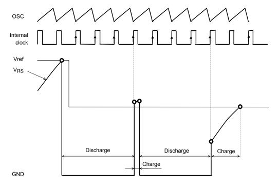
Transition from discharge mode to charge mode
