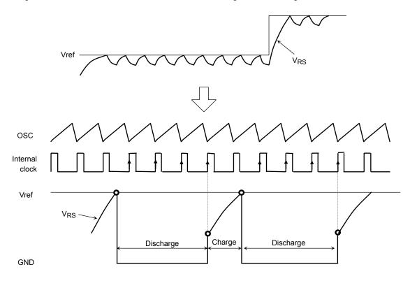
Transition from charge mode to discharge mode
