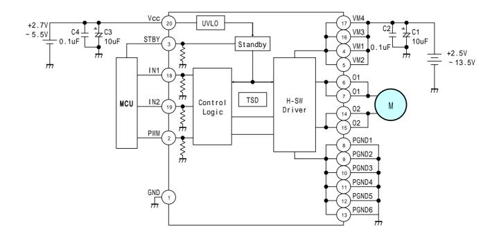
Note : The power supply capacitor should be connected as close as possible to the IC.
