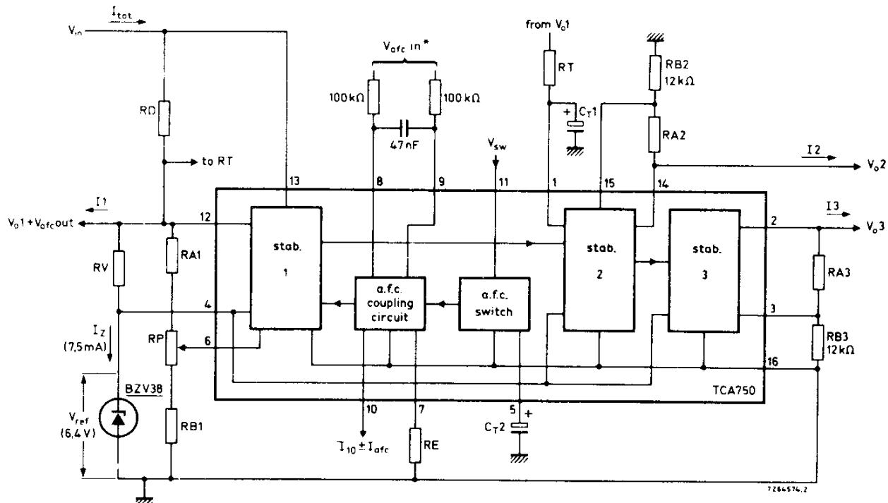
\*  $V_{afc}$  is superimposed on a common-mode voltage ( $V_{com}$ ) of 5 V to 17 V.
