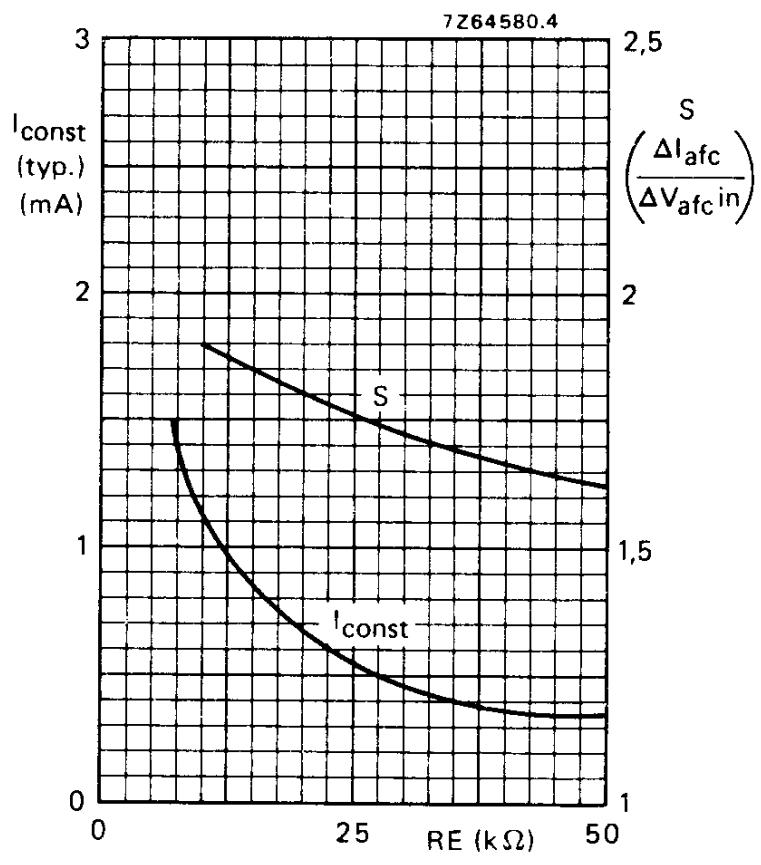
Fig. 5 Determination of  $I_{10}$  and S-factor ( $S$  = a.f.c. slope) from  $RE$ .
