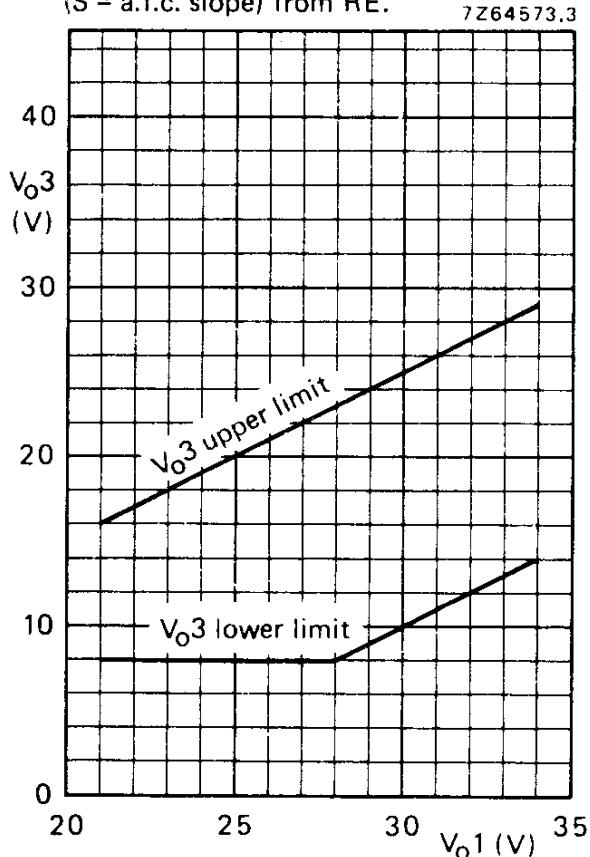
Fig. 7 Range of values for  $V_{o3}$ .
