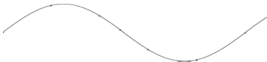
Typical waveform at speaker inputs after LC filtering
