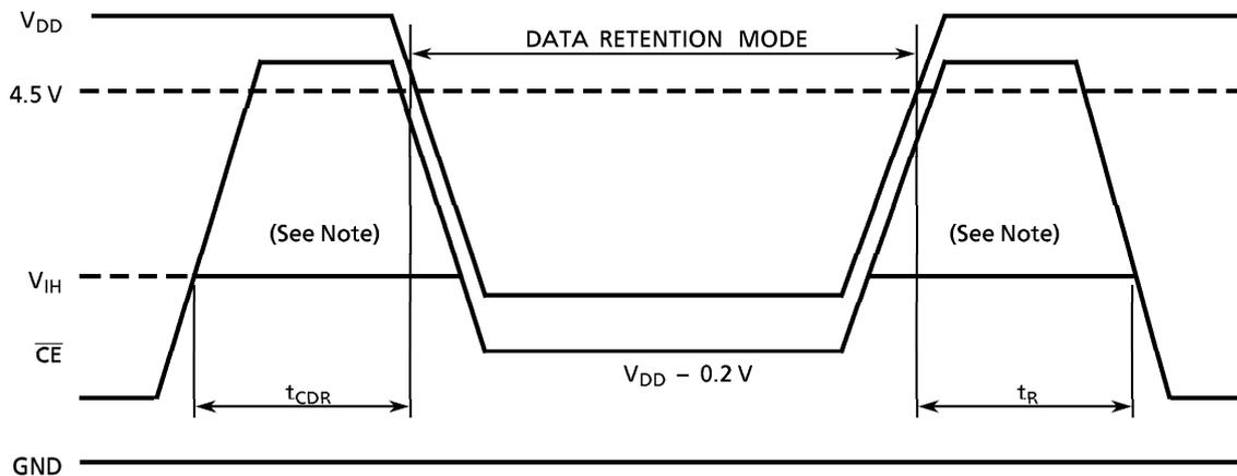
Note: When  $\overline{CE}$  is operating at the V<sub>IH</sub> level (2.2 V), the standby current is given by I<sub>DDs1</sub> during the transition of V<sub>DD</sub> from 4.5 to 2.4 V.
