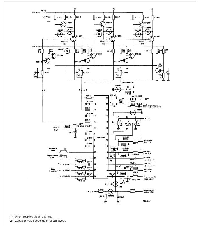
Fig.3 Typical application circuit diagram using the TDA3507.
