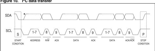
Figure 10. I<sup>2</sup>C data transfer
