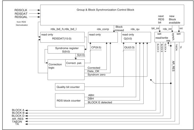
This module is used to acquire group and block synchronization of the received RDS data stream, which is provided in a modified shortened cyclic code. For theory and implementation of modified shortened cyclic code and error correction, please refer to CENELEC Radio Data System (RDS) specification EN50067.
