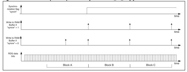
The RAM buffer is used as a circular FIFO (Figure 9). If more than 24 blocks are written, the oldest data will be overwritten. One level of the buffer consists of 4 bytes (2 information bytes, 2 RDS data bytes). If less than 4 bytes of the RAM buffer are read out from the master via the SPI or I<sup>2</sup>C interface, the buffer address will not be incremented.
