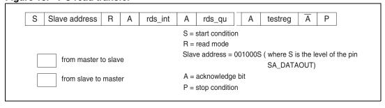
13 bytes can be read at a time (please refer to Section 3.8 for the meaning of each bit).
