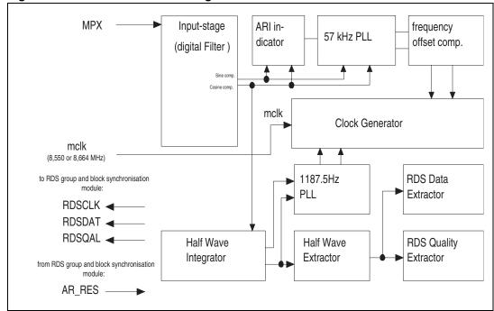
Figure 4. Demodulator block diagram
