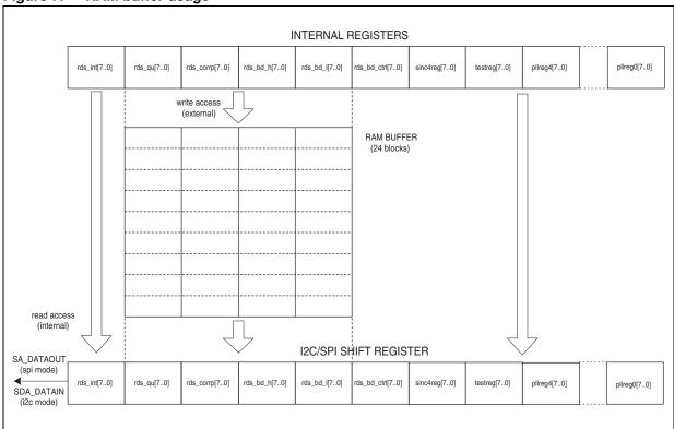
After power up, or after resynchronization by setting "ar\_res" rds\_int[5] to one, incoming RDS blocks are stored in the RAM buffer when synchronization has been established (*Figure 8*). But if the bit "syncw" rds\_bd\_ctrl[0] (refer to *Section 3.8.6*) is cleared, every received RDS block is stored, also without synchronization. This means if the RDS is not synchronized, every received consecutive 26 RDS data bits are treated as a RDS block.
