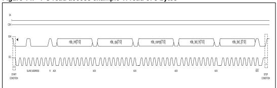
Figure 15. I<sup>2</sup>C read access example 2: read of 1 byte
