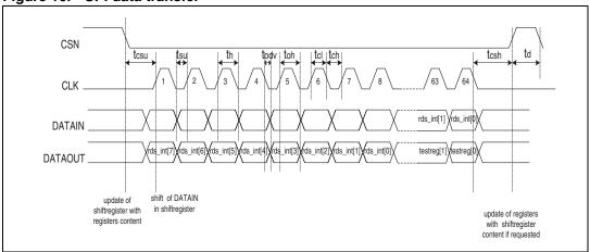
This interface consists of four lines (*Figure 16*). A serial data input (DATAIN), a serial data output (DATAOUT), a chip select input (CSN) and a bit clock input (CLK).
