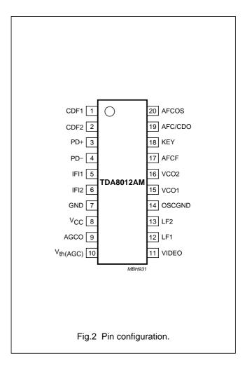
The circuit provides an AGC signal which is used to drive a gain-controlled IF amplifier (TDA8011T or TDA8010AM) for a stable PLL demodulation characteristic.
