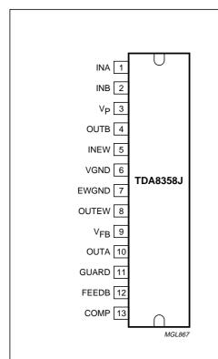
The die has been glued to the metal block of the package. If the metal block is not insulated from the heatsink, the heatsink shall only be connected directly to pin VGND.
