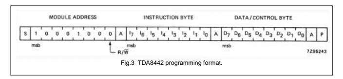
Acknowledge (A) is generated by the TDA8442 only when a valid address is received and the device is not in the power-down-reset mode ( $V_P > 8.5 \text{ V (typ.)}$ ).
