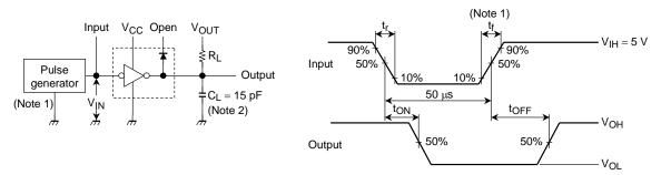
Note 1: Pulse Width 50  $\mu s,$  Duty Cycle 10% Output Impedance 50  $\Omega,$   $t_{f}$   $\leq$  5 ns,  $t_{f}$   $\leq$  10 ns
