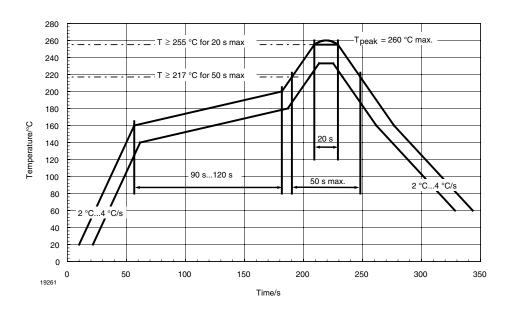
Figure 2. Solder Profile, RSS Recommendation
