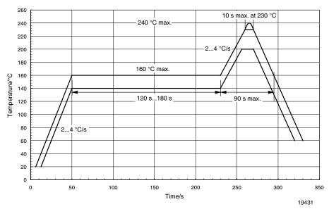
Figure 1. Recommende Solder Profile for Sn/Pb soldering.
