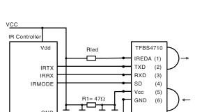
Figure 3. Recommended Application Circuit
