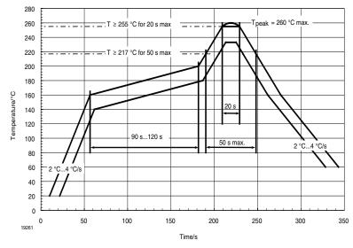
Figure 4. Solder Profile, RSS Recommendation
