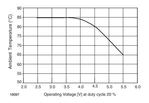
Figure 6. Temperature Derating Diagram
