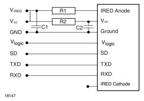
Figure 1. Recommended Application Circuit
