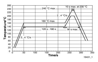
Figure 3. Recommended Solder Profile for Sn/Pb soldering
