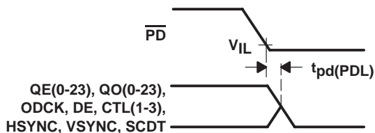
Figure 7. Delay From \overline{PD} Low to Hi-Z Outputs
