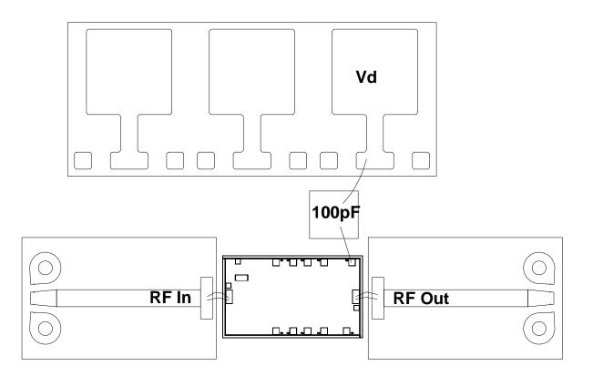
All DC connections may be brought in from either side of the chip (Use Pad 6 or 8) 0.01uF external Cap is recommended on Drain Bias: Vd = 5V (Id = ~80mA)
