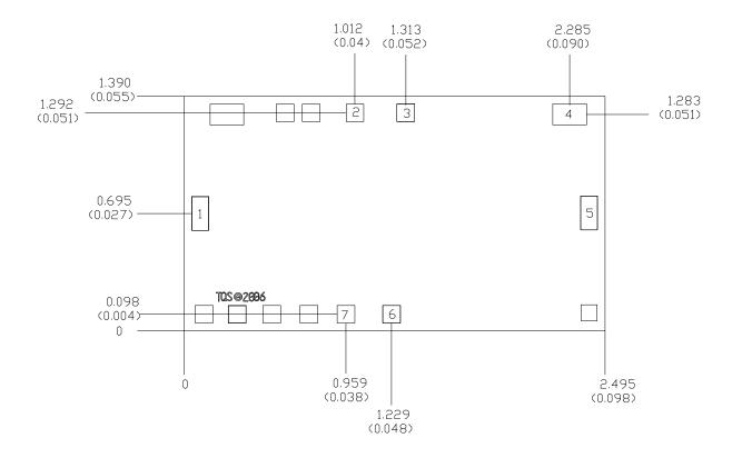
Units: millimeters (inches) Thickness: 0.1016 (0.004) (reference only) Chip edge to bond pad dimensions are shown to center of Bond pads. Chip size tolerance: +/- 0.0508 (0.002) RF Ground through Backside
