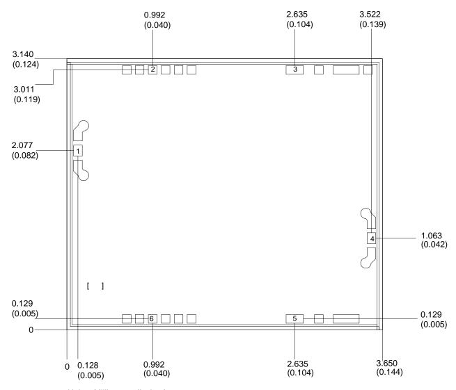
Units: Millimeters (inches) Thickness: 0.100 (0.004)
