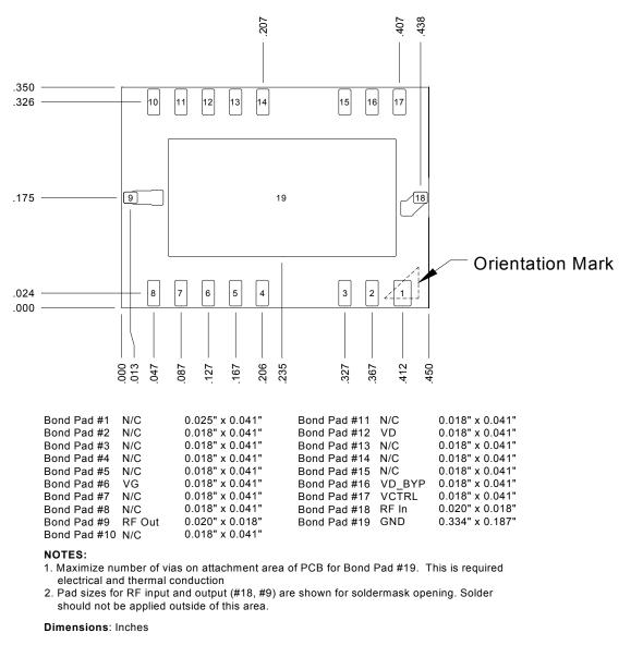
Tolerances: Length & Width: ±0.003" Height: ±0.006" Adjacent Pad to Pad Spacing: ±0.0002" Pad Size: ±0.001"
