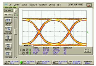
Input Signal Vin = 1V<sub>PP</sub> Includes 8GHz Bessel Filter
