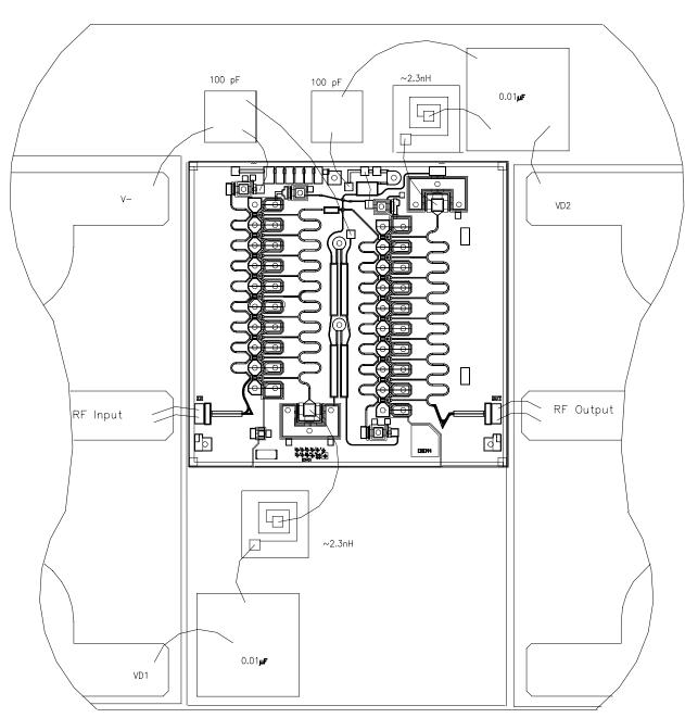
RF connections: Bond using two 1.0-mil diameter, 20 to 30-mil-length gold bond wires at both RF Input and RF Output for optimum RF performance.
