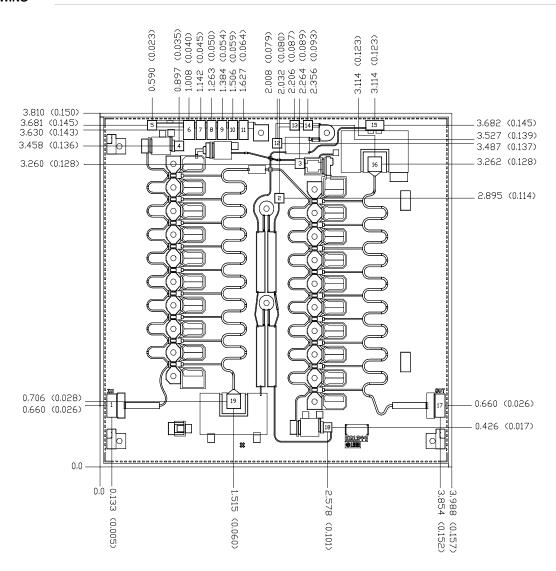
Units: millimeters (inches) Thickness: 0.1016 (0.004)
