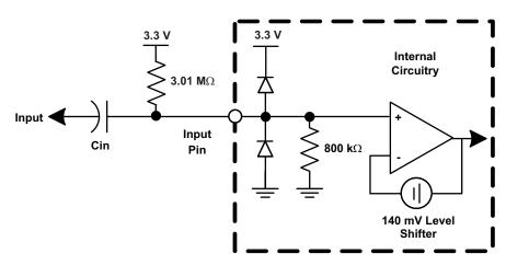
Figure 30. AC-Bias Input Mode Circuit Configuration
