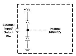
Figure 26. Internal ESD Protection
