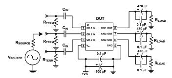
Figure 3. AC Coupled Input and Output Test Circuit
