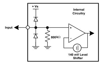
Figure 28. Equivalent DC Input Mode Circuit
