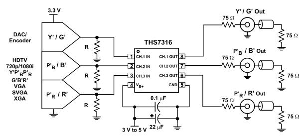
Figure 31. Typical HDTV Y'P'<sub>B</sub>P'<sub>R</sub> / G'B'R' System with DC-Coupled Line Driving
