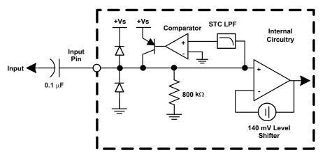
Figure 29. Equivalent AC Sync Tip Clamp Input Circuit
