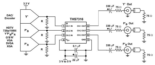
Figure 27. Typical HDTV Y'/P'<sub>B</sub>/P'<sub>R</sub> Inputs From DC-Coupled Encoder/DAC With AC-Coupled Line Driving
