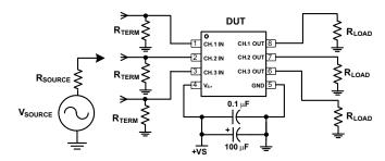
Figure 2. DC Coupled Input and Output Test Circuit
