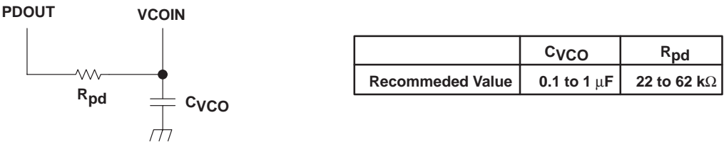
Figure 8. Resistor and Capacitor Connection
