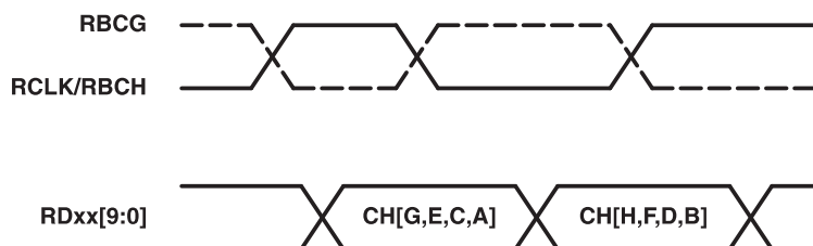
Figure 6. Multiplexed Channel Receive Timing
