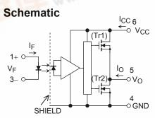
A 0.1- $\mu$ F bypass capacitor must be connected between pins 6 and 4. (See Note 6.)
