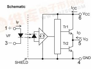
0.1  $\mu F$  bypass capacitor must be connected between pins 6 and 4. (Note 4)
