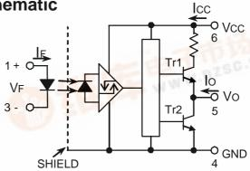
0.1uF bypass capacitor must be connected between pin 6 and 4
