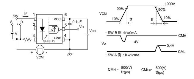
CM<sub>L</sub> (CM<sub>H</sub>) is the maximum rate of rise (fall) of the common mode voltage that can be sustained with the output voltage in the low (high) state.
