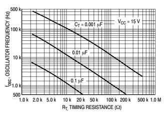
Figure 3. Oscillator Frequency versus Timing Resistance
