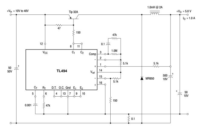
Figure 21. Pulse Width Modulated Step-Down Converter
