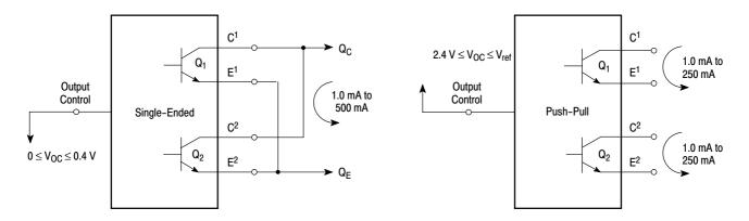
Figure 17. Output Connections for Single-Ended and Push-Pull Configurations
