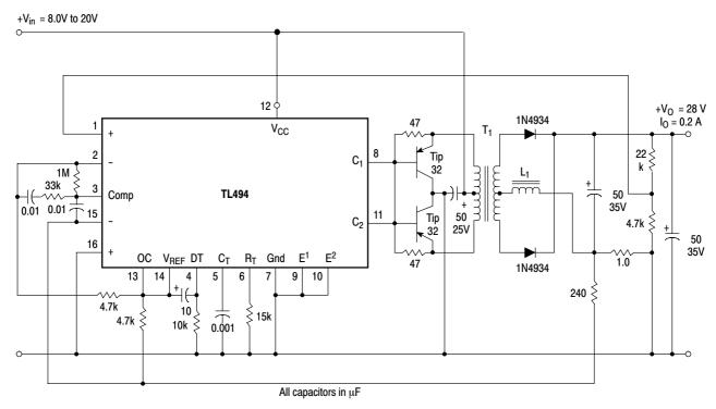
Figure 20. Pulse Width Modulated Push-Pull Converter
