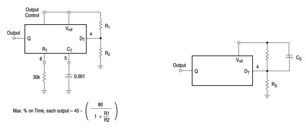
Figure 15. Deadtime Control Circuit
