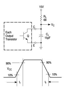
Figure 12. Common–Emitter Configuration
