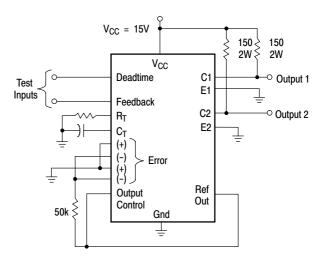
Figure 11. Deadtime and Feedback Control Circuit
