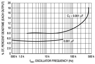
Figure 5. Percent Deadtime versus Oscillator Frequency
