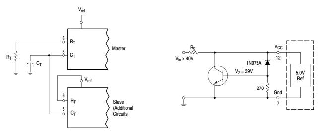
Figure 18. Slaving Two or More Control Circuits
