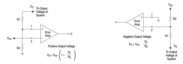
Figure 14. Error-Amplifier Sensing Techniques
