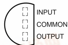
TL750L... LP PACKAGE (TO-92, TO-226AA) (TOP VIEW)
