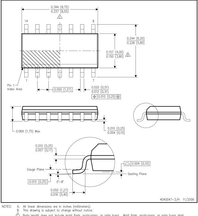
Body length does not include mold flash, protrusions, or gate burrs. Mold flash, protrusions, or gate burrs shall not exceed .006 (0,15) per end.
