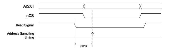
Tie to L for the CPU's where nCS is enabled and addresses are valid after the read signal goes low.
