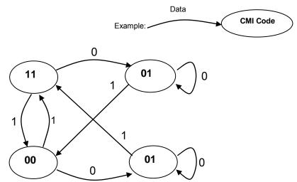
Figure 10 - CMI Coding State transition diagram
