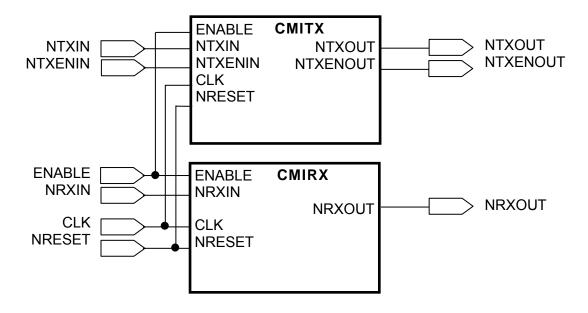
Figure 11 - CMI Modem Block Diagram
