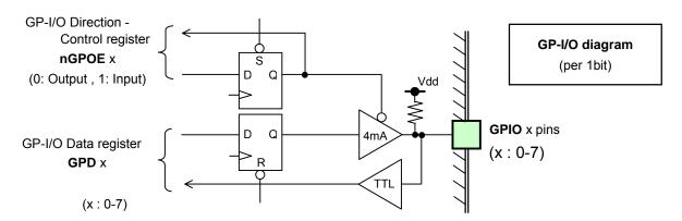
Two registers, named "Direction control register" and "Data register", are added for the GP-I/O control. To allocate these registers in COMR7 (Address=0Eh), the sub address is enhanced by one bit (SUBAD3).
