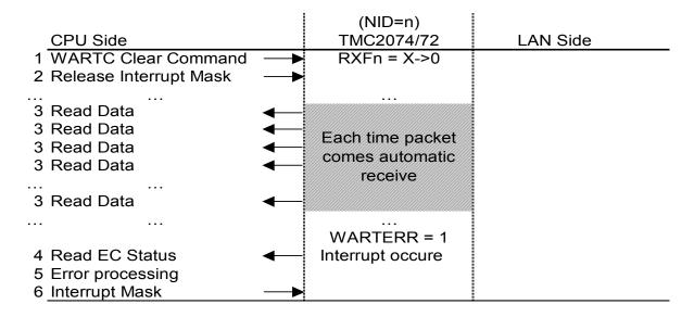
After completing the receive of remote buffer mode, RRCV (Remote buffer receive end flag) in the EC interrupts the status register (INTSTA) and changes from 0 to 1, permitting the flag to be an interrupt source. This mode also monitors if a packet comes from applicable nodes within a certain period. If there is a non-responsive node, the WARTERR flag changes from 0 to 1, permitting this change to be an interrupt source. Refer to section 3.2.10 - INTSTA Register: EC Interrupt Status.
