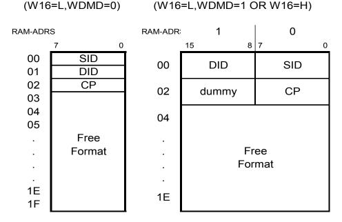
Figure 8 - Packet Structure of Free Format Mode (Example of 32 bytes/page)
