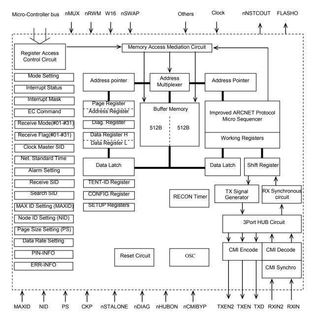
Figure 1 - TMC2072 Internal Block Diagram
