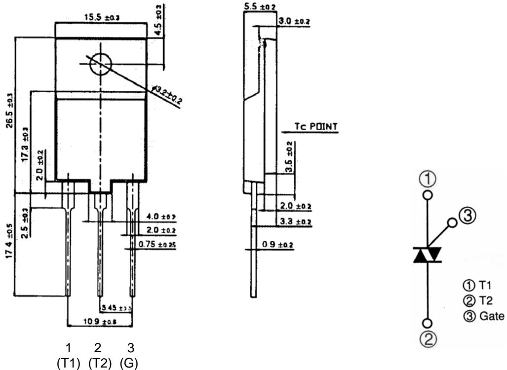
\* Dimensions in millimeters (1mm=0.0394")
