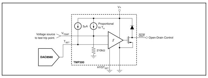
Figure 11. DAC Generates the Voltage-Driving T<sub>SET</sub> Pin
