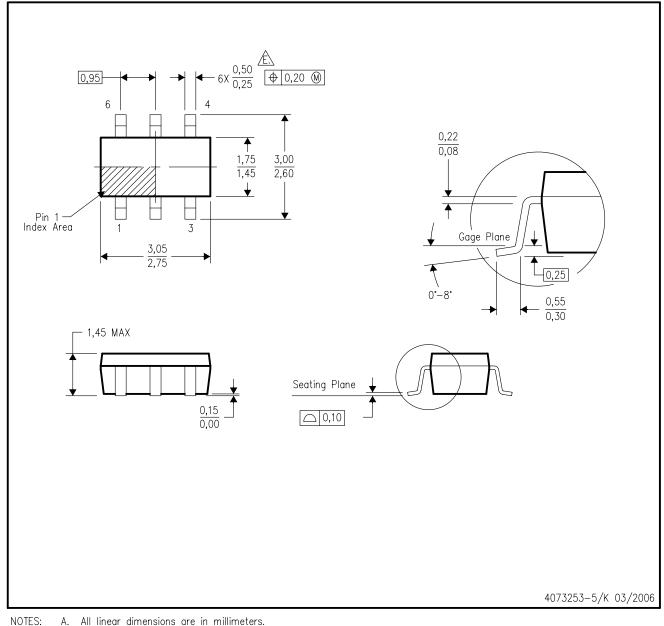
A. All linear dimensions are in millimeters.
