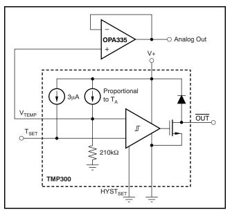
Figure 9. Buffering the Analog Output Signal
