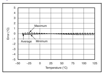
Figure 12. 5°C Hysteresis Error vs Temperature
